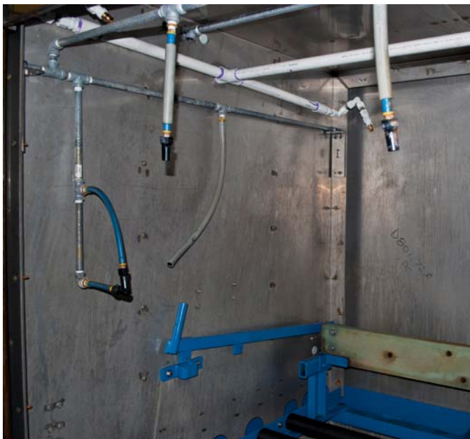
One piece PVC piping manifold will not corrode and clog nozzles
