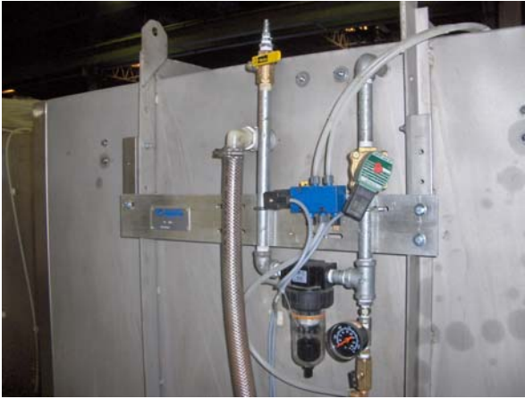
Solenoid mounting plate in new position
