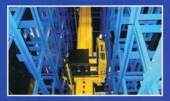
5. The battery management system instructs the ASRS system to take the discharged battery from the staging area to the proper charge location.
