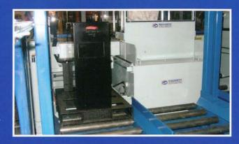
2.) The Super-Xchanger deposits the discharged battery in the battery staging area.
