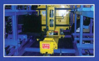
6.) The battery management system instructs the ASRS system which battery to return to the staging area.
