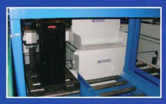
The Super-Xchanger picks up a charged battery from the staging area.
