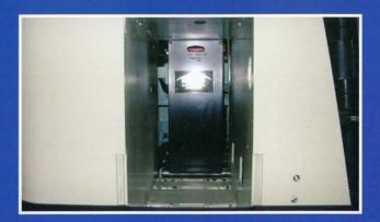
1.) The battery management system identifies the battery and lift truck as it enters the change out area. The Super-Xchanger extracts the battery from the lift truck.
